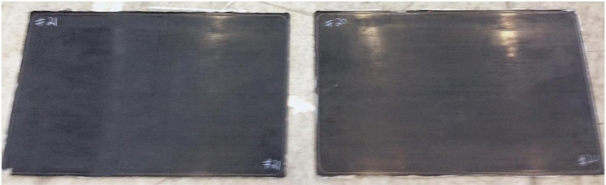
Figure 3 – Comparison recycled to virgin fiber molded panels; panel orientation matches that of Figure 2.
