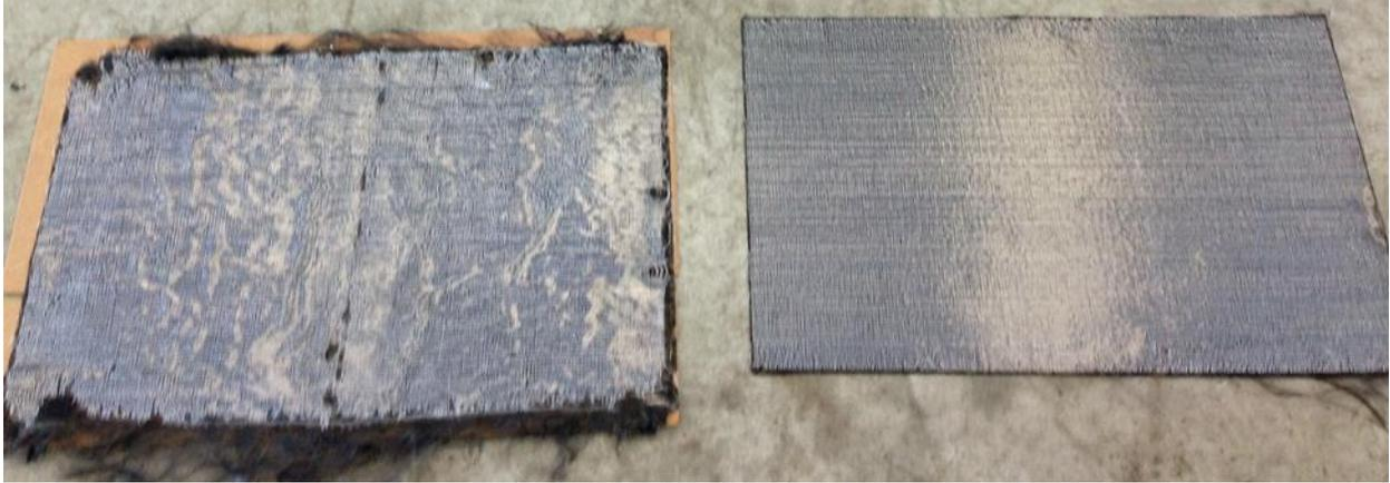
Figure 2 – Recycled and virgin fiber preforms just prior to resin infusion
