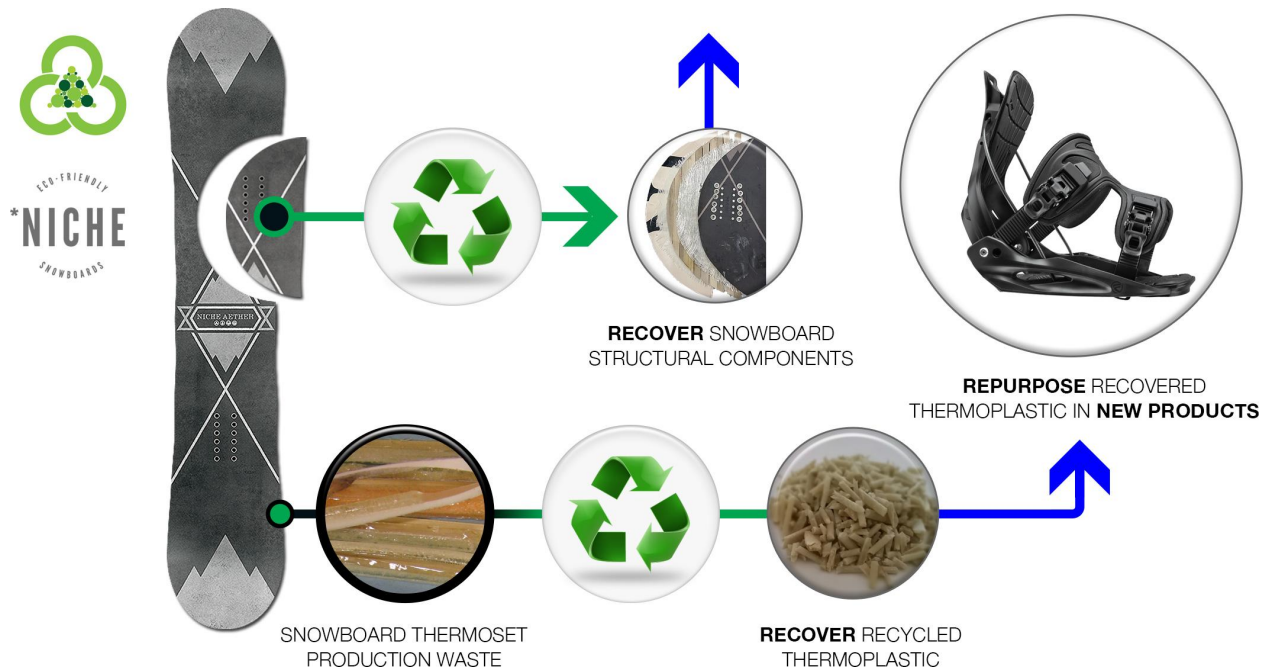
Figure 2. Recyclamine thermoset technology allows manufacturers to design fully recyclable products, and recycle & repurpose thermoset manufacturing waste back into thermoplastic products.
