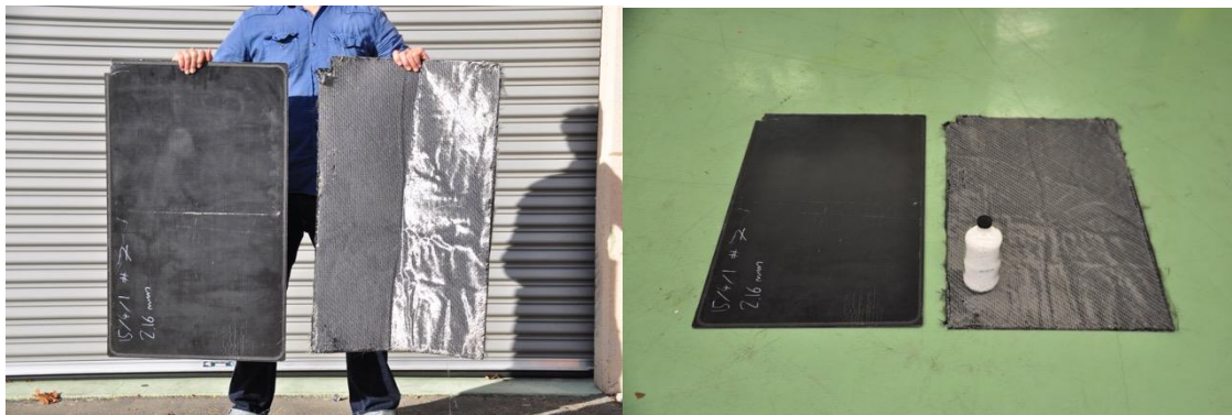
Figure 3. Recyclable carbon fiber composites made with Recyclamine ® Technology. Automotive panels before & after recycling. Carbon fiber can be recovered and reused to make another panel (not shown).
