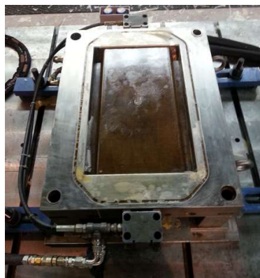
Figure 3 Omega shaped mold used for HPRTM specimen manufacturing
