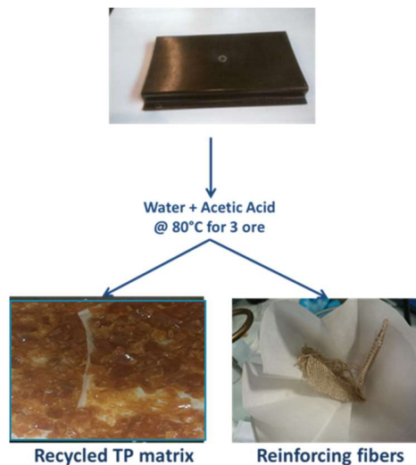
Figure 6 Scheme of chemical recycling and resulting products
