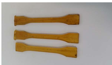
Figure 8 Dog bone specimens produced by injection molding of the recovered thermoplastic obtained from the chemical recycling of the epoxy network of cured laminates
